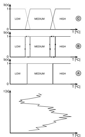
Fig. 3. Conversion the values of diagnostic signals to the statement values based on: (A) – threshold; (B) – hysteresis function; (C) – fuzzy sets;
